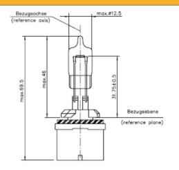
Light center length: 31,75mm ± 0,5mm Bulb diameter: max. 12,5mm
